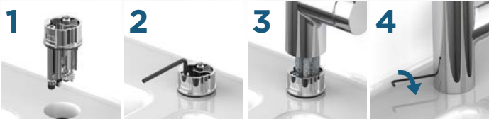
1 Drop the base 2 Secure to the deck 3 Fit body on the base 4 Secure the body to the base
